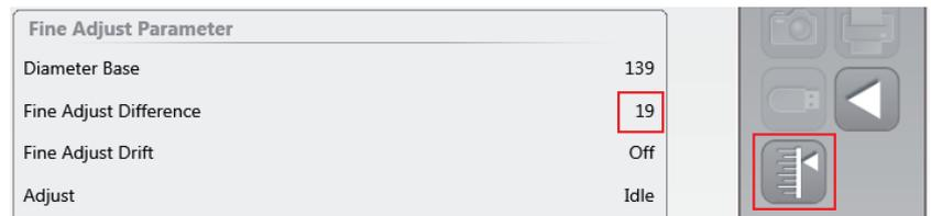
A single spindle adjustment should be performed when a sensing head of a current group is replaced or a large diameter deviation ( $> \pm 10\%$ ) was determined for a spindle.
