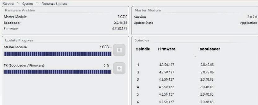
The screenshot shows the 'Firmware Update' window after a successful update. Both progress bars, 'Master Module' and 'TK (Bootloader / Firmware)', are now at 100%. The 'Spindles' table on the right shows updated firmware and bootloader versions for all spindles.
