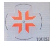
1. Touch the first calibration point (top left) with a fine, non-scratching object until the next calibration point is displayed (the display changes from TOUCH to HOLD to RELEASE).
